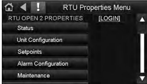
Fig. F — RTU Properties Menu Screen
